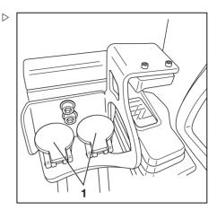
Plug connectors on the lift mast
