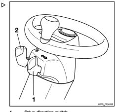
1 Drive direction switch 2 Turn indicator switch
