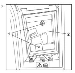
Remove any dust and dirt from the fresh-air ▷ inlet (1) beneath the filter mat carrier.
