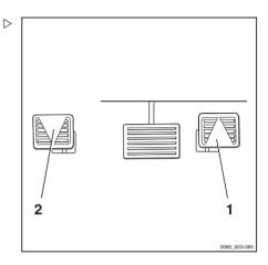
The indicator for the selected drive direction ("forwards" (1) or "reverse" (2)) lights up on the display-operating unit.
