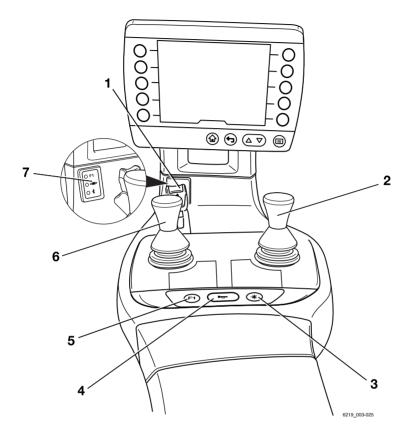
Drive direction switch 1 Cross lever "Attachments"
