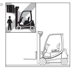
Lower the load until it rests securely on the prack.
