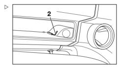
Using the hexagon socket wrench, turn the emergency lowering screw (3) a maximum of 1.5 revolutions to loosen it.
