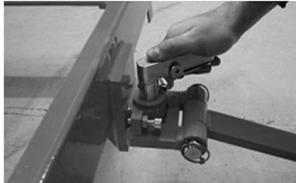
– Evenly tighten the clamping bolts on the hinged tiller (**tightening torque: 30 Nm**) and secure the clamping bolts with nuts (**tightening torque: 50 Nm**).
